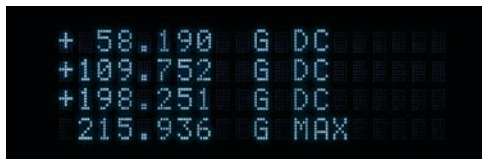
Max DC Hold On —the display configured to show the live DC field readings for the X, Y, and Z axis, as well as the maximum field reading (settable to any axis)
