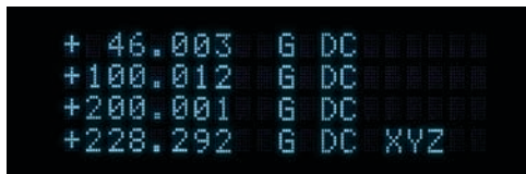
Normal Reading —the display configured to show the live DC field readings for the X, Y, and Z axis, as well as the vector magnitude
