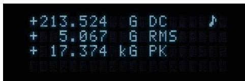
3 Separate Probe Readings On —the display configured to show the X, Y, and Z axis as three separate gaussmeters: the X axis as a DC field reading with audible and visual alarm, the Y axis as an RMS field value, and the Z axis as a peak field value
