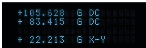
Differential Reading On —the display configured to show the live DC field readings for the X and Y axis, as well as the X-Y axis differential reading
